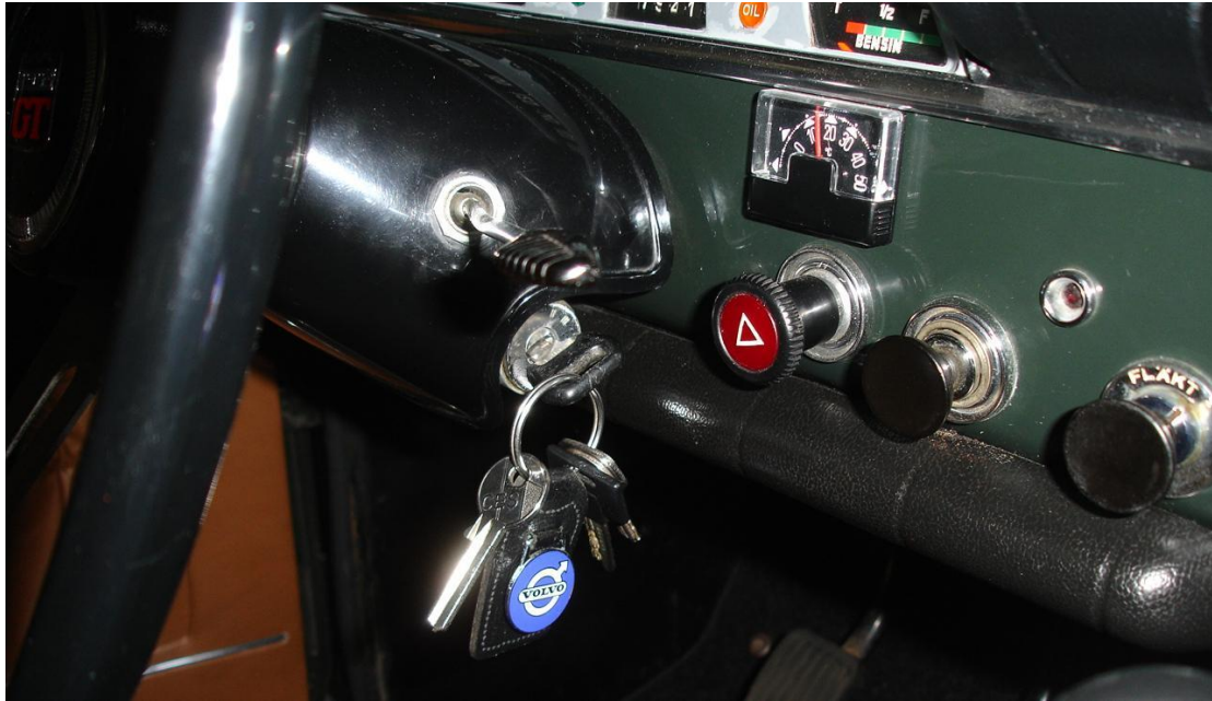
Emergency flasher unit, 1969 123 GT (part number unknown)
