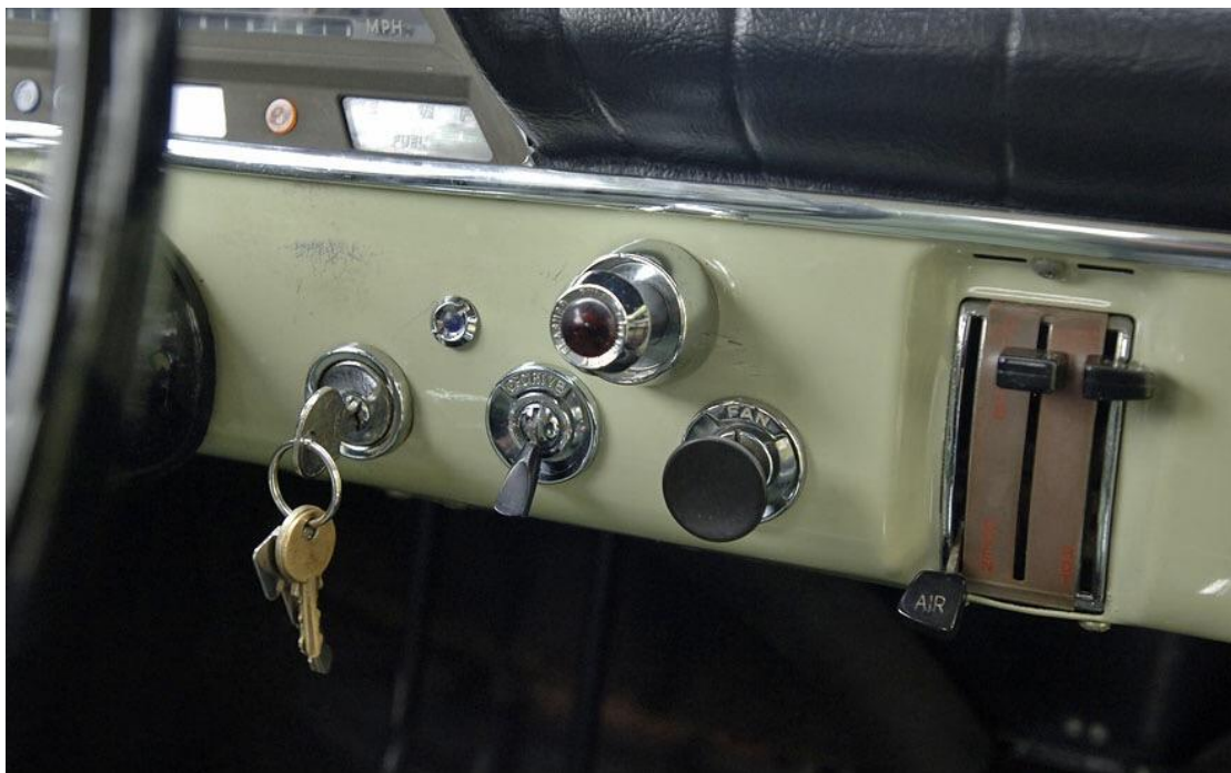
Emergency flasher unit, 1966 122 s (part number unknown)
