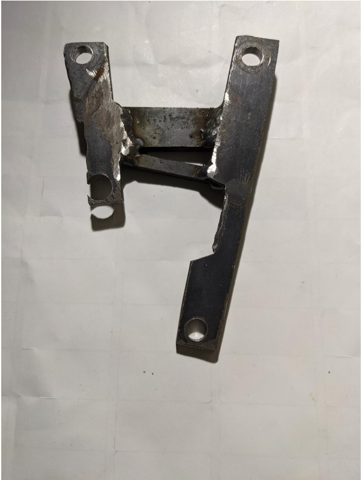
Prototype of the mounting bracket for screwing it into the electric servo in the lower holes and screwing the upper holes into the front bracket for steering axle (which seems / may have been added in 1969 and I had to manufacture it as there wasn't any the 68)
