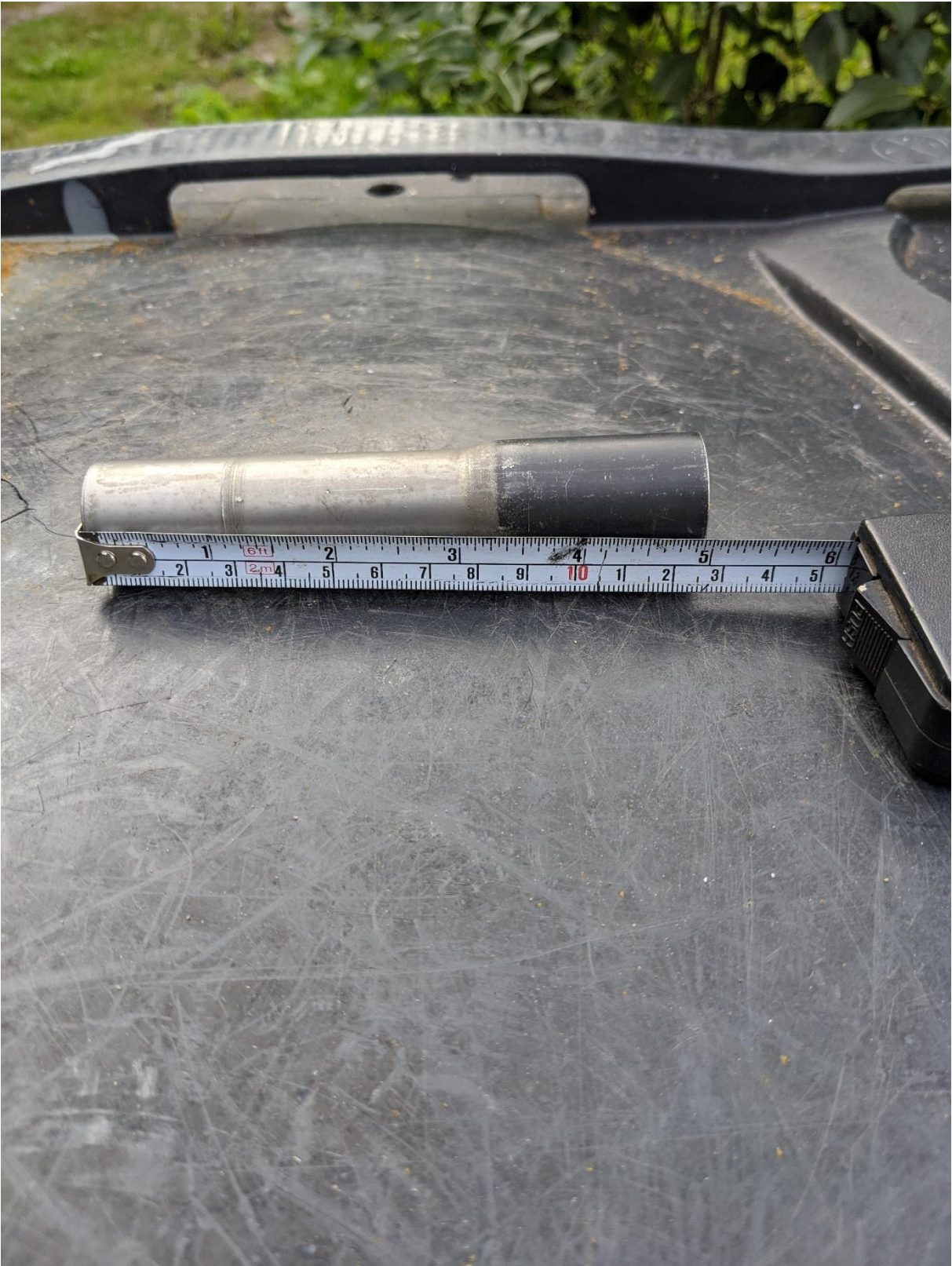
Upper axle from Toyota cut at the top of the bulge on the way up to the steering wheel.
