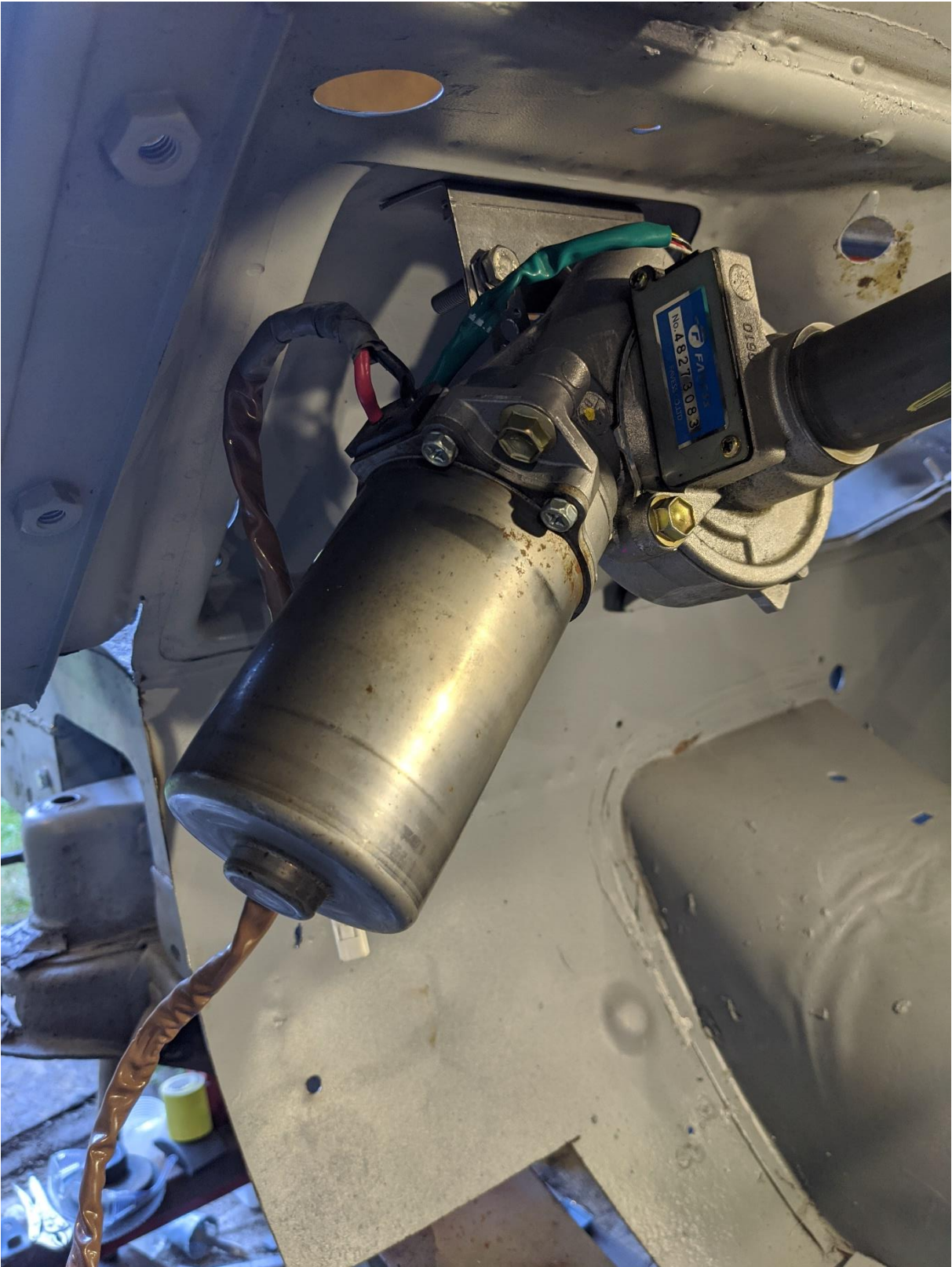
As there was no front bracket for steering axle on the 68, one was made and screwed in place after I took measurements on the 69
