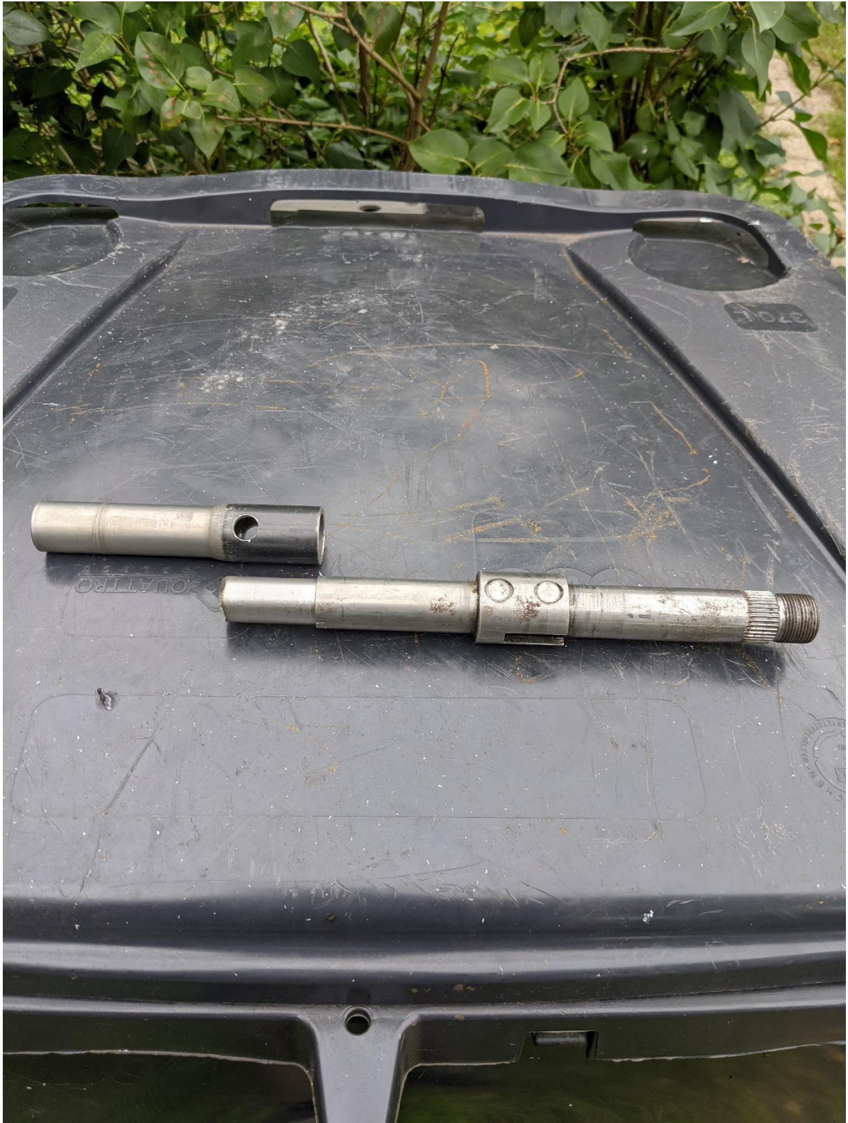
Upper axle from Toyota, cut and turned upper steering axle from Amazon Total length of these pieces assembled and welded is 330mm
