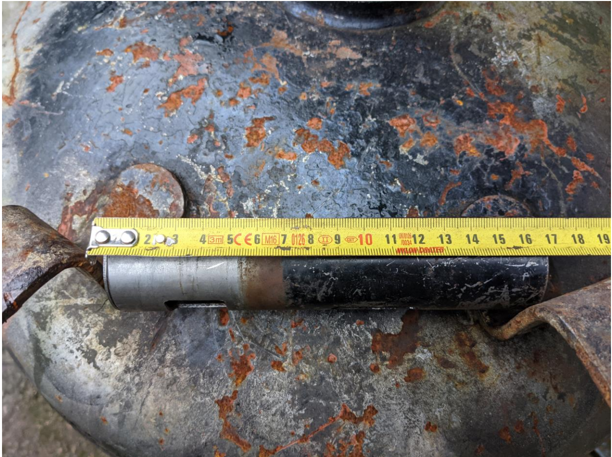
Amazon upper outer steering tube cut, now 165mm long
