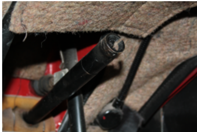
10.1 Fit output shaft through bulkhead
