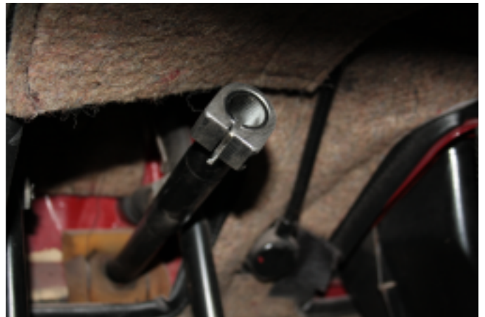
10.2 Fitting the clamp on the shaft
