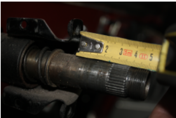
6.1 Measuring the shaft
