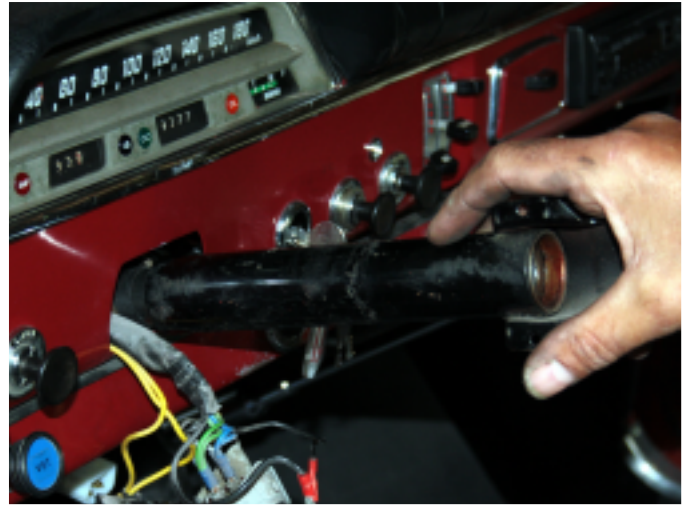
13.2 Refitting steering shroud
