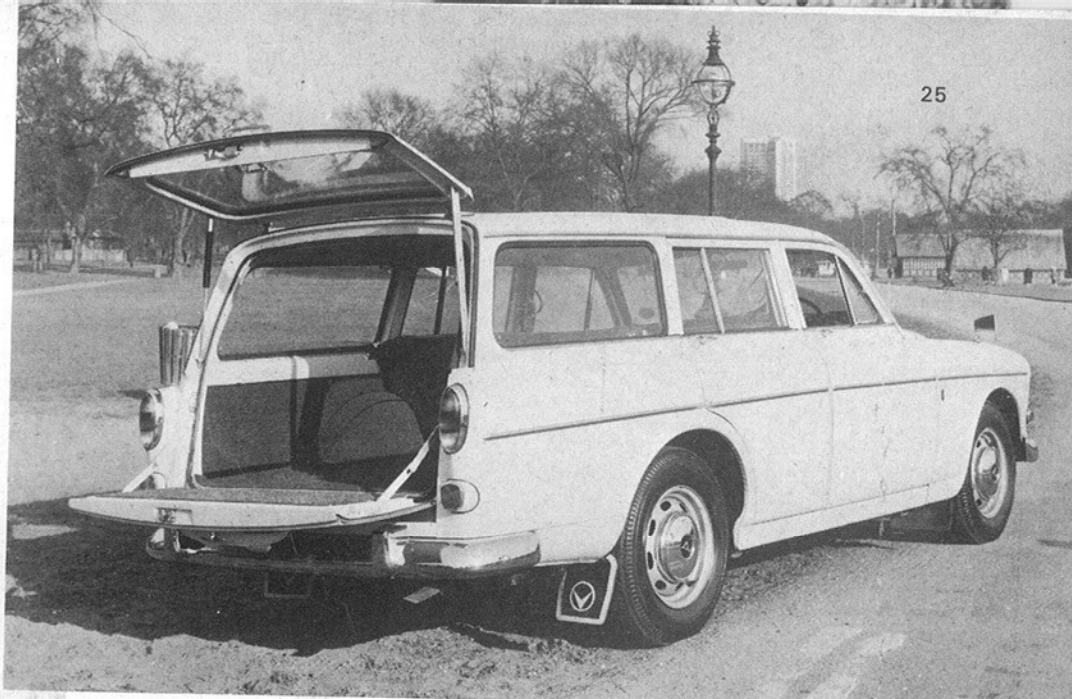
Estate car body has clean lines. Upper door is automatically raised when lower door is opened and held by a strut with a spring of compressed gas.
