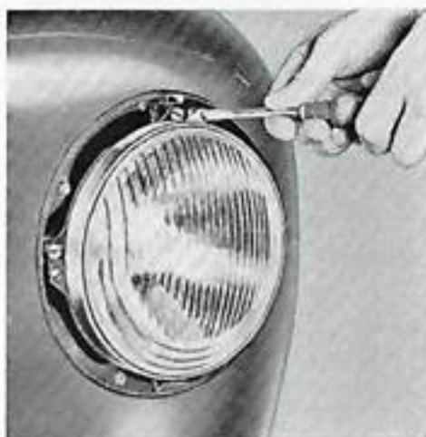
3. Loosen the three screws retaining the insert.
