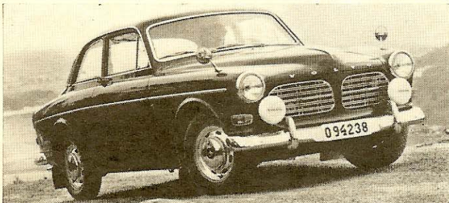
123 GT has 115-bhp engine, new grille texture and radial tires.
